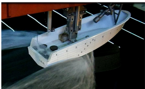
Towing tank trial
